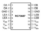
Note: Input disable mode not available on RC73687 SOIC package.
